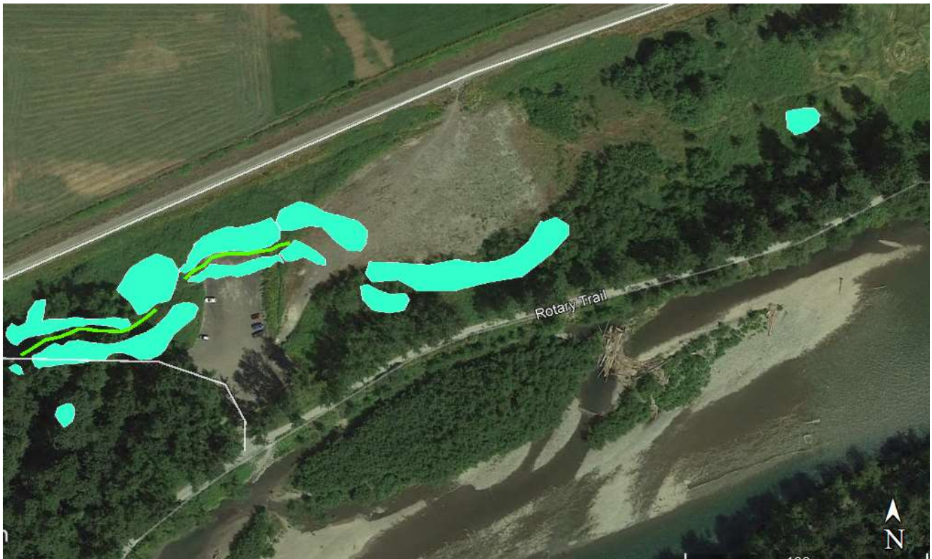
Figure 3 Replanting Area resulting in 3,648m 2 . Turquoise polygons show where potted stock and live stakes are mixed together. Green lines show dense cluster plantings of willow stakes to help shade the waterway and provide leaf litter.
